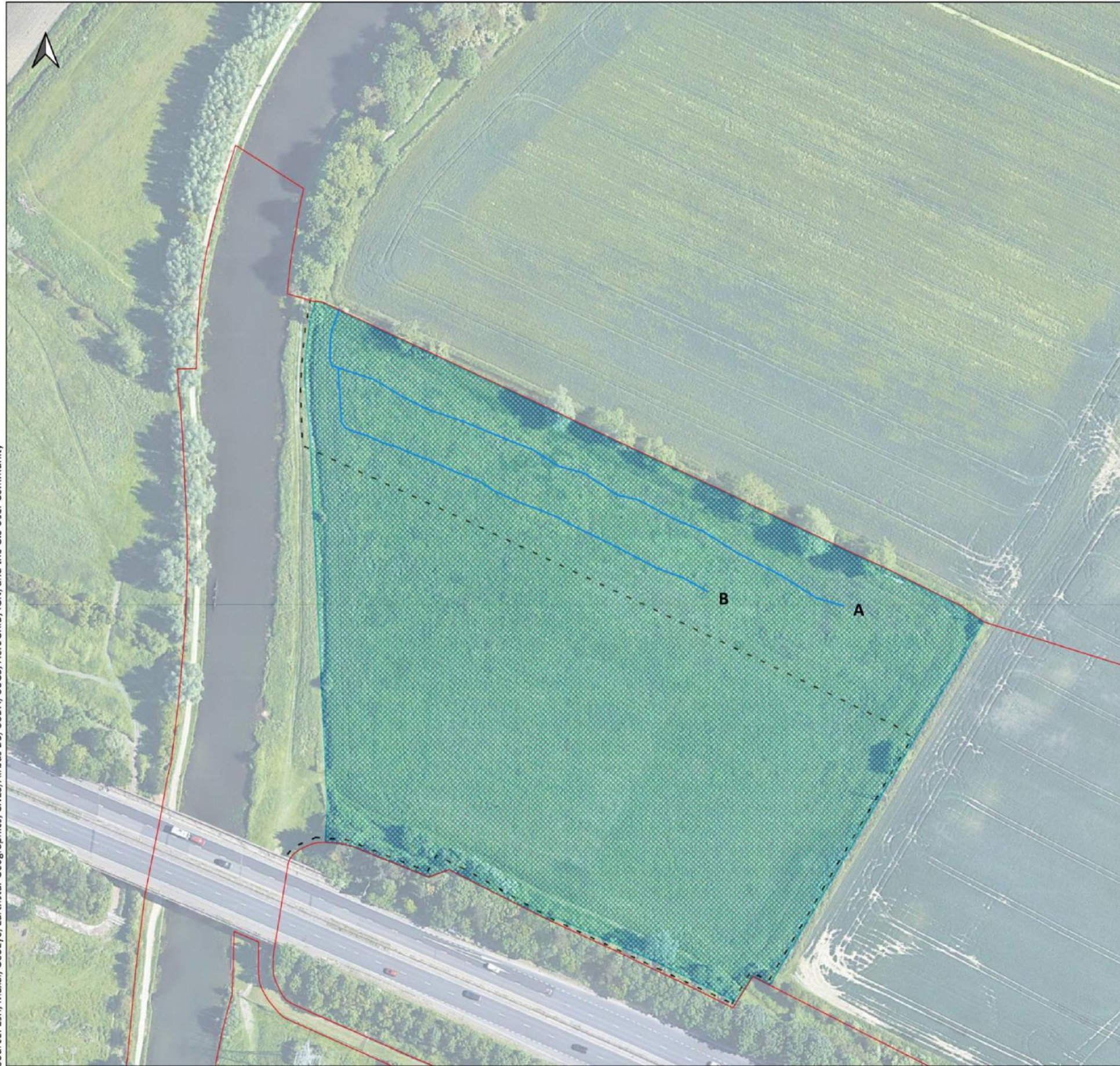
Figure 1 Indicative Alignment of Proposed Ditch Features
